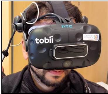
Figure 4: For the VR study a HTC Vive head-mounted device with built-in eye tracking from Tobii and Leap Motion sensor was used.
