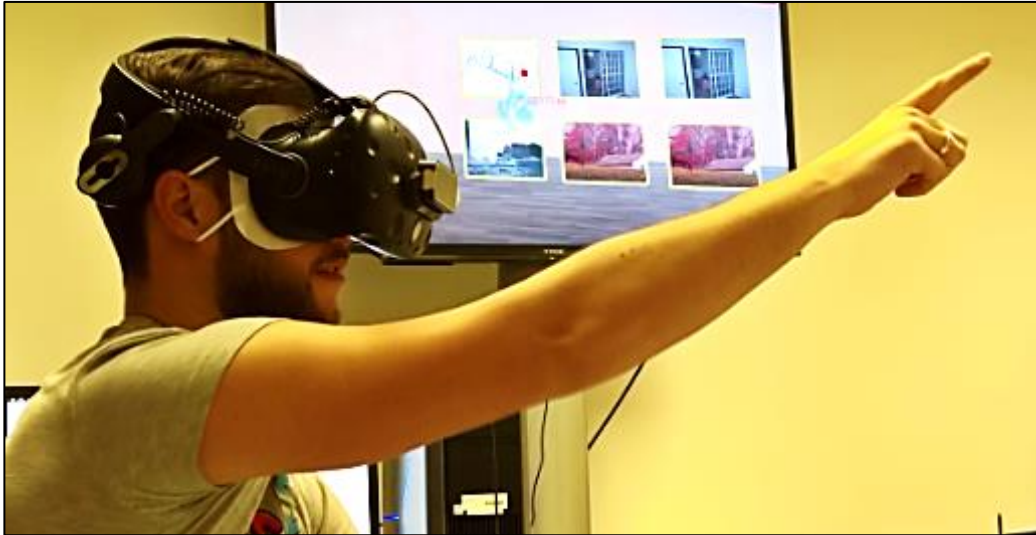
Figure 1. Measurement of emotion using VR technology with built-in eye tracking and analysis of gaze behavior towards selected stimuli of an affective image database [9]. Participants manually select image pairs in a concentration game while gaze (red point on operator display) is tracked.
