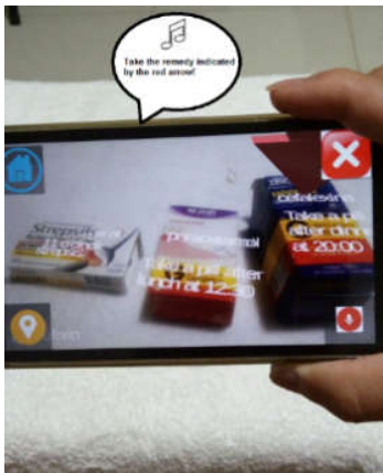
Figure 1. The app reminds and identifies for the individual with AD or the caretaker, the correct medicine box indicated by a red arrow sign and with a spoken alert.
