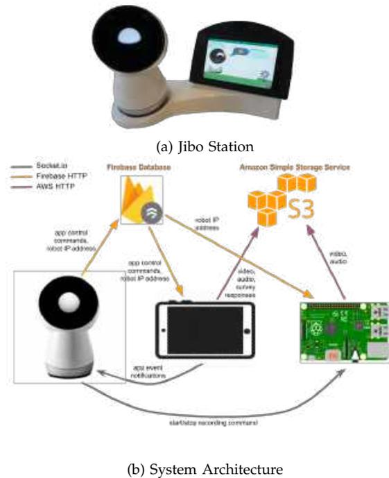
Fig. 1: A portable station that integrates a Jibo robot, a tablet and a Raspberry Pi with an USB camera.
